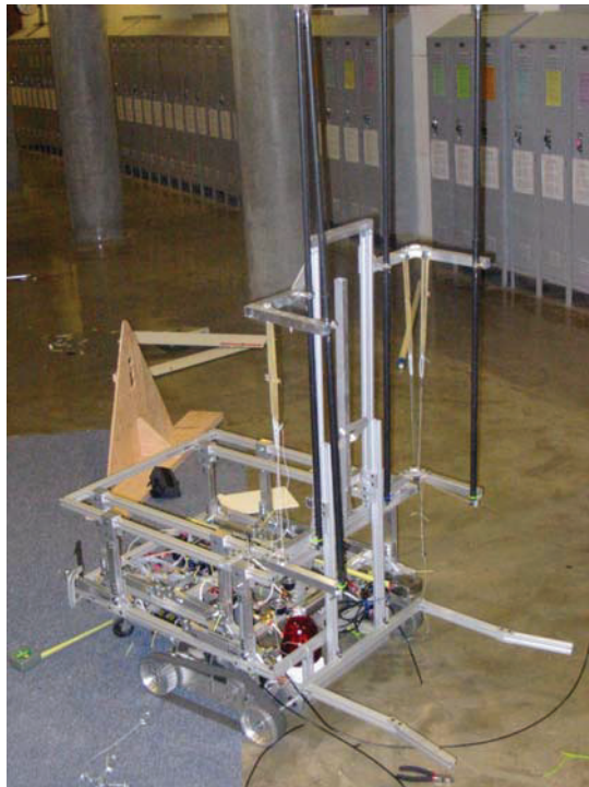
Fig. 11. The robot with the box manipulation system extended during testing. Pneumatic pistons were used to extend the rails of the box manipulation system.
